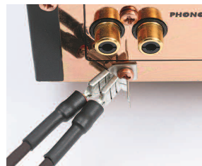
Figure 5, Showing two grounding wires connected to the chassis tag
