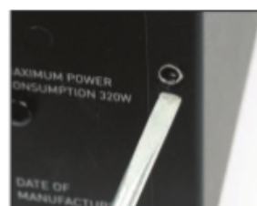
Remove the screw and scratch a small area of paint off with a screwdriver
