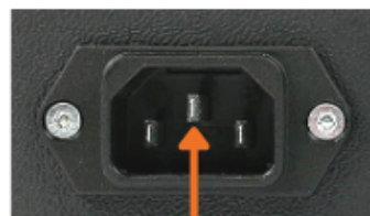
Earth pin on IEC socket
