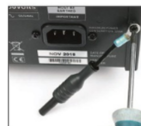
Attach the Chassis Ground Adaptor and screw back in
