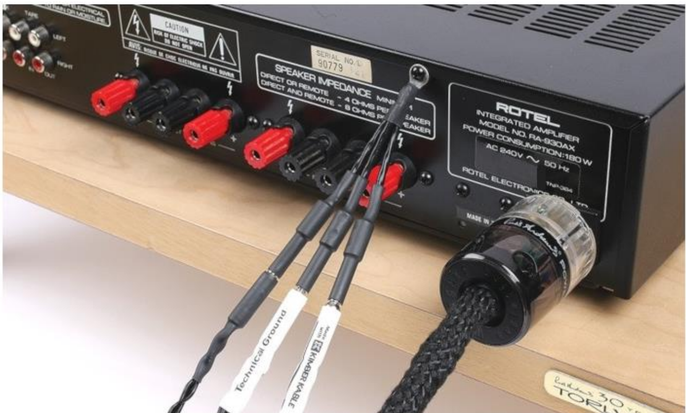
Image shows grounding cables connected to the chassis of a Rotel amp via a 3-way Chassis Ground Banana Adaptor.
