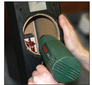
In our case the backing plate can be released more easily if you soften the plastic clips attaching it to the casing
