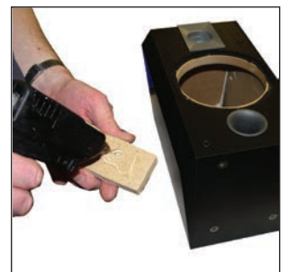
Apply hot melt glue to the insulation board
