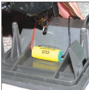
When you are happy with the value of capacitor you have used, fix it in position with hot melt glue and reassemble your speakers
